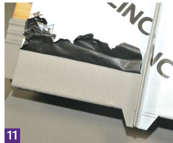
11 The film must not be partially removed as this can cause staining.
