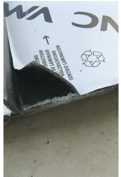
Partial removal of protective film.
