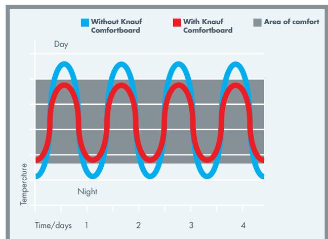
Optimised room temperature through active climate control: latent heat accumulator compensates for peak temperatures.
