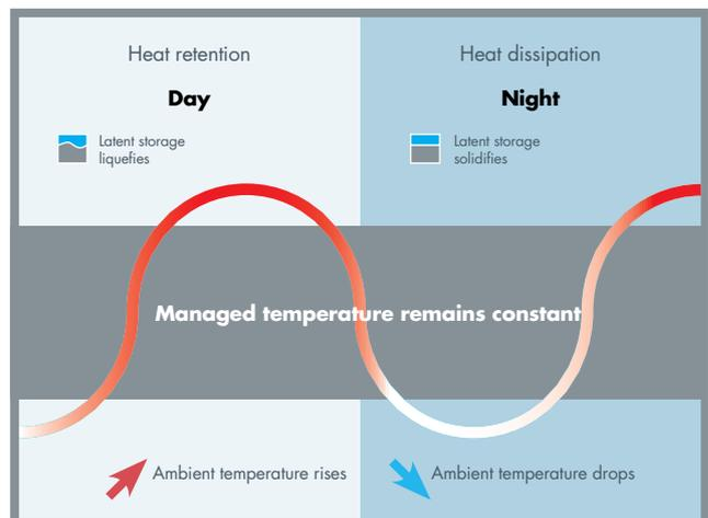
The principle of latent heat accumulator work.
