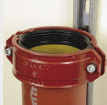
2. Push coupling over the end of the pipe or fitting ensuring the central register is abutted against the spigot edge.
