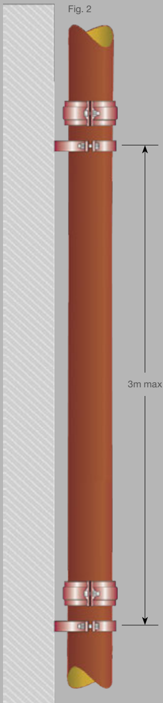
Typical support arrangement for vertical pipework.
