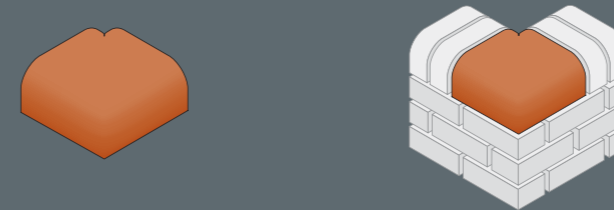
BN.19 External return to double bullnose on edge and to Bullnose Double Header on Flat (square corners on bed)
